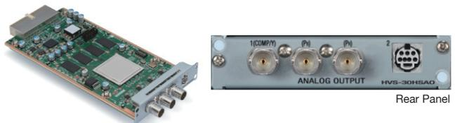
The analog output card provides 2 analog outputs. These can be set up as composite, component or one of each. Of course the composite output is down converted in HD mode.
