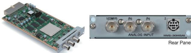
The analog input card provides 2 analog inputs. These can be set up as composite, component or one of each.
